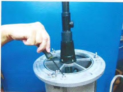
Figure 21: Removal of allen screw
