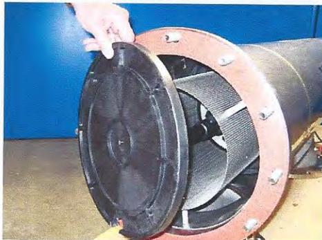
Figure 12: Removal of prestrainer cap.
