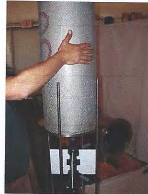
Figure 24: Screen removal
