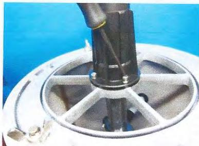
Figure 23: Remove reverser housing screws
