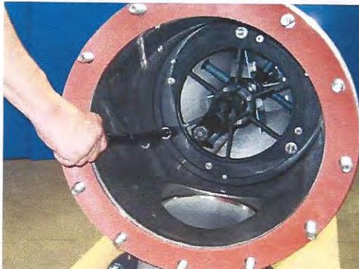
Figure 15: Loosening clamp nuts
