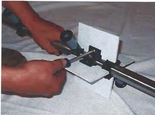
Figure 30: Removing the rotor paddles
