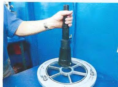
Figure 23a: Remove reverser housing
