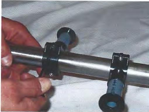
Figure 32: Nozzle removal
