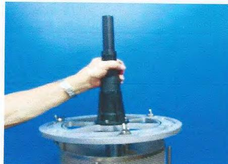
Figure 22: Upper bulkhead removal
