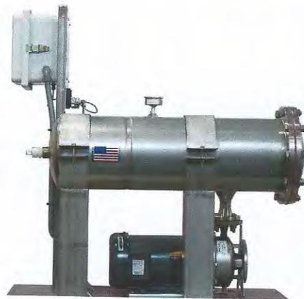
Figure 2: Saddle-type filter support
