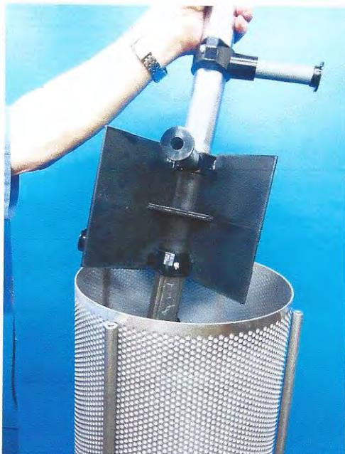
Figure 26: Rotor removal
