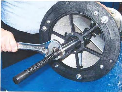
Figure 28: Removal of the retaining nut
