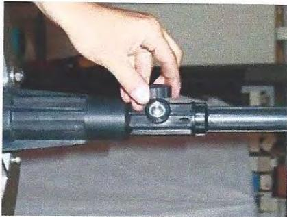
Figure 19: Removing pawl retainer cap
