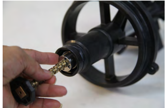
Figure 16 Final installation of pawl and reverser
