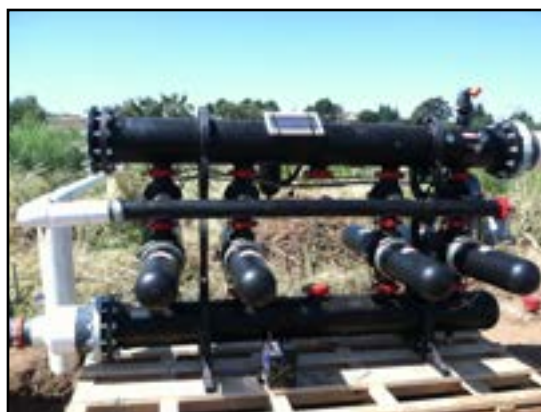
Figure 2. Example of a Netafim Apollo Disc-Kleen Filter
