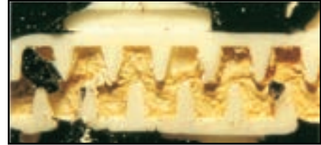
Figure 5. Dripper with calcium precipitate. The black pieces in the picture are pieces of the cut-away plastic dripline and not contaminants.
